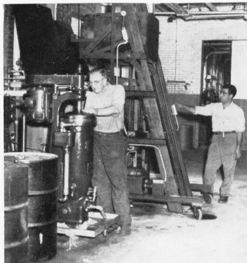
(1) Vincenzo Cinquegrana (right) controls the flow of used oil into a "settling" tank where water, acid, sludge and foreign materials drop to the bottom. The oil, which remains on the top, is siphoned into a centrifuge (Hugh McColl sets gauge) where any remaining water is separated. It then goes through a filter to remove any possible dirt particles, and finally into a storage tank.
