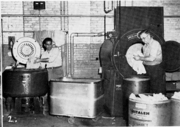
A spinner removes excess water and the wash then goes into the drier (2). Hugh takes out dried wash from the dryer to make way for the "spun" wash which Vincenzo removes from the spinner.
